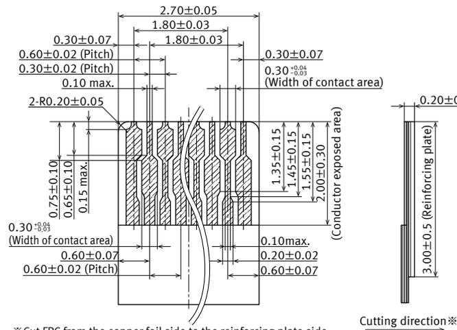
※ Cut FPC from the copper foil side to the reinforcing plate side.
