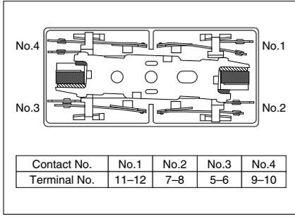
The table below shows the state of the other contacts when the current through the welded form "a" contact is 0 V and the rated voltage is applied through the form "b" contact.
