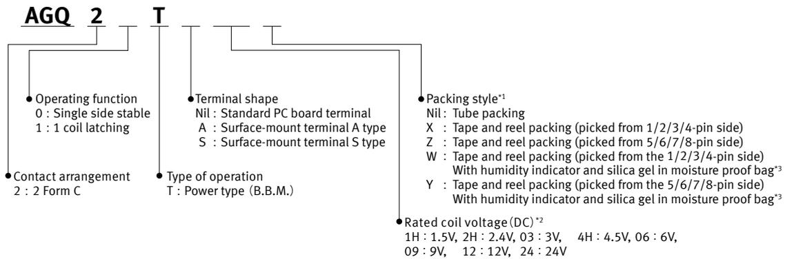
\*1. The "W" and "Y" at the end of the part number only appears on the inner and outer packing. It does not appear on the relay itself.
