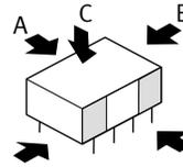
Please chuck the
