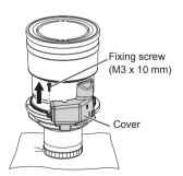
Remove the one fixing screw (M3 x 10 mm) from the cover.
