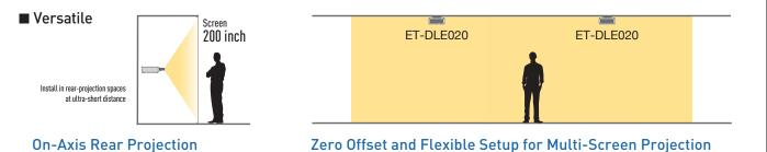
The ET-DLE020's straight mirrorless design makes screen-centered projector installation possible in rear-projection applications. Note: Hot spots may occur depending on the screer
