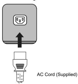
Plug the connector in to the display unit.
