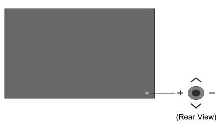
**To turn on the Display:** Press the centre of the joystick in and hold it down for a few seconds, the Display will turn on.
