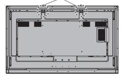
1 Remove the eyebolt cap from the eyebolt mounting position (two locations).
