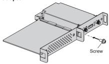
• Tightening torque guideline: 0.6 N·m or less
