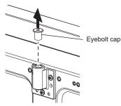
2 Attach the eyebolt to the mounting position (two locations).
