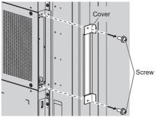
**5** Insert the function board to the main unit slot, and fix it with the 2 screws removed in step 4.
