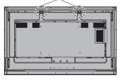
1 Remove the eyebolt cap from the eyebolt mounting position (two locations).
