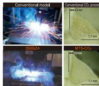
• Joint: Fillet • Base Metal: Mild Steel SPCC (I2.3 mm/120 A)
