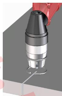
Attach the finger guard to the shield cup so that the opening is always positioned opposite to the cutting direction as shown in the figure on the left.
