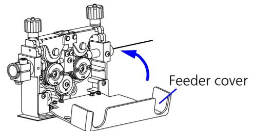
(12) Straighten the welding torch and feed forward the wire by pressing the inching switch on either remote controller or operation panel of the welding power source.
