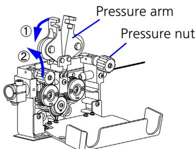
(10) Adjust the pressure nut so that the bottom of the pressure nut is positioned within the scale range of the applied wire.
