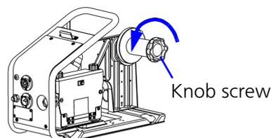
(2) Remove the knob screw from the spool shaft.
