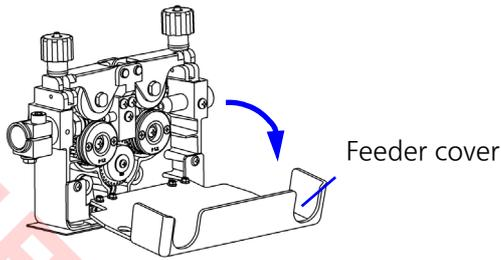
(6) Pull the both pressure nuts forward, and then lift up the pressure arm.
