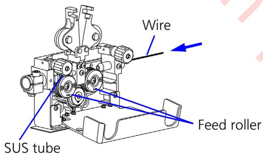
(9) Pull down the pressure arms and set the pressure nuts back in place.
