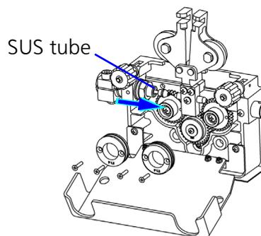
(5) Fix the feed roller with the flat head machine screw so that the wire size indication of the applied wire is shown in the front.
