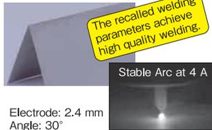
The recalled welding parameters achieve high quality welding.
