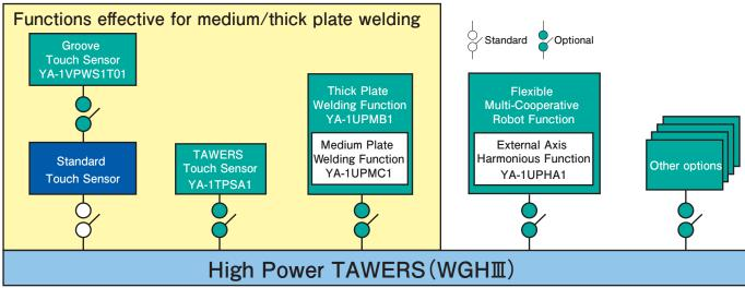
Note: Touch Sensor Software and Wire Clamp Unit are supplied with TAWERS for Medium and Thick Plates.
